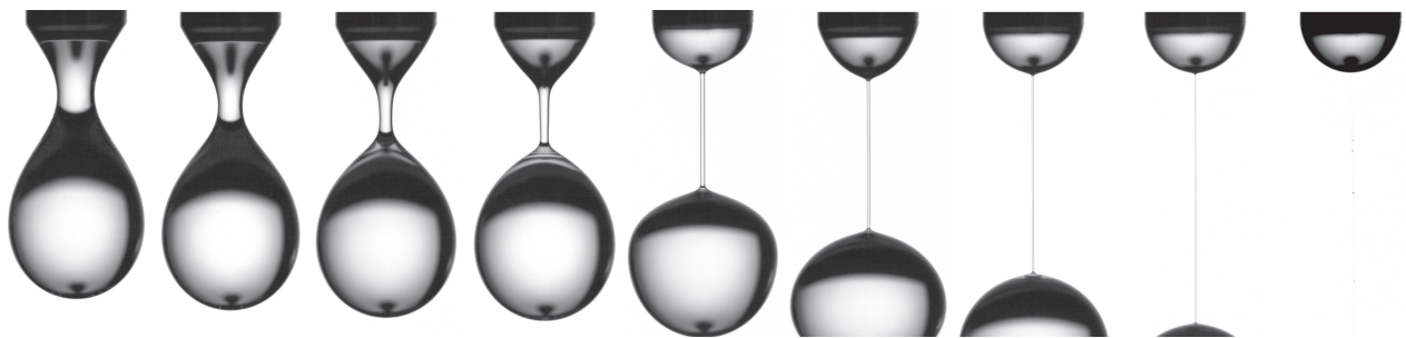
Figure 1: Extension, thinning and pinch-off of a droplet of aqueous solution of polyethylene oxide (PEO). The nozzle is 2.75mm-wide.
