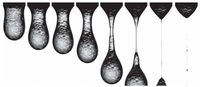
Detachement of a drop of a granular suspensions of polystyrene beads (250 µm-big) in silicone oil. The nozzle is 2.75 mm-wide. As the drop falls, the neck thins down following different dynamics depending on how its size relates to the cooperative length.
